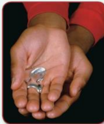
Figure 2.4 Physical Change The silvery substance in the photograph is gallium, which has a melting point of 30^{\circ}\text{C} . Infer What can you infer about the temperature of the hand holding the gallium?
