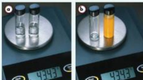
Figure 2.16 Conservation of Mass When the liquids in a , are mixed, they react. The products are shown in b . None of the products are gases. Analyze Data How do you know that a reaction took place and that mass was conserved during the reaction?
