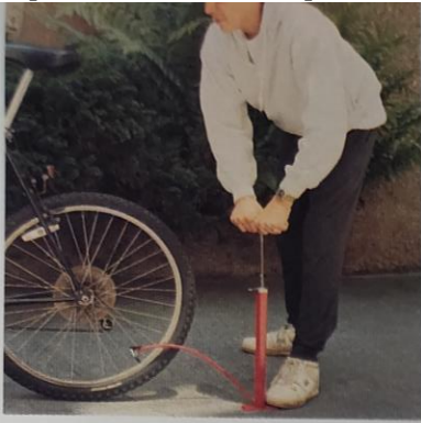
Figure 24.3 ▲ Do work on the pump by pressing down on the piston and you compress the air inside. Adiabatic compression—the air is warmed.
