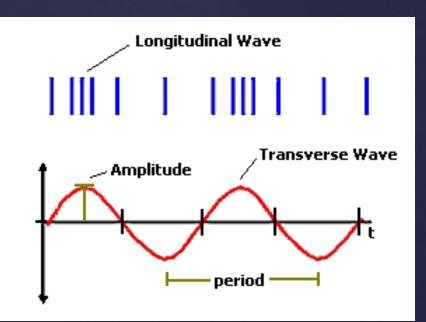
When a tuning fork vibrates, it creates areas of high pressure (compressions) and low pressure (rarefactions). As the tines of the fork vibrate back and forth, they push on neighboring air particles. The forward motion of a tine pushes air molecules horizontally to the right and the backward retraction of the tine creates a low-pressure area allowing the air particles to move back to the left.
