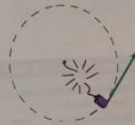
Figure 9.7 ▲ When the string breaks, the whirling can moves in a straight line, tangent to—not outward from the center of—its circular path.
