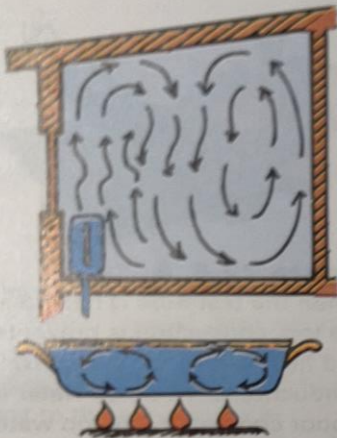
Figure 22.6 ▲ (Top) Convection currents in air. (Bottom) Convection currents in liquid.
