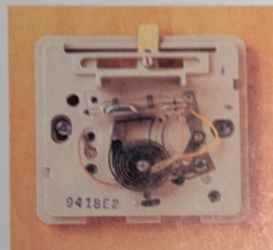
Figure 21.11 ▲ A thermostat. When the bimetallic coil expands, the mercury rolls away from the electrical contacts and breaks the circuit. When the coil contracts, the mercury rolls against the contacts and completes the electric circuit.
